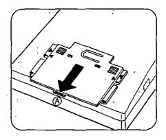
Removing the card holder: Push the card holder in the direction of arrow "B" while keeping the tip of the holder pulled in the direction of arrow "C", to take off the holder.
