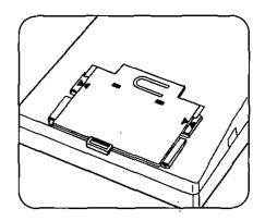
Push two shaded portions slightly and insert the edges of the holder under the slide rails and then slide down in direction of arrow "A".
